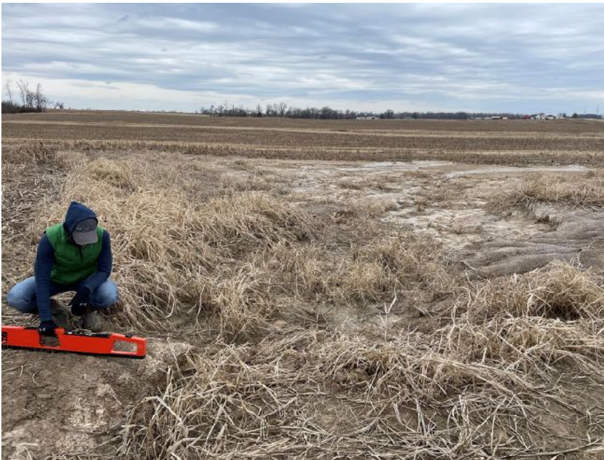
Photo 1: Mindy on Site 2 using the EM 38 on an eroded hillslope
