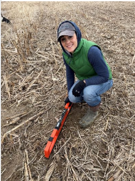
Photo 3: Mindy collecting conductivity readings in adjacent non-affected cropland.
