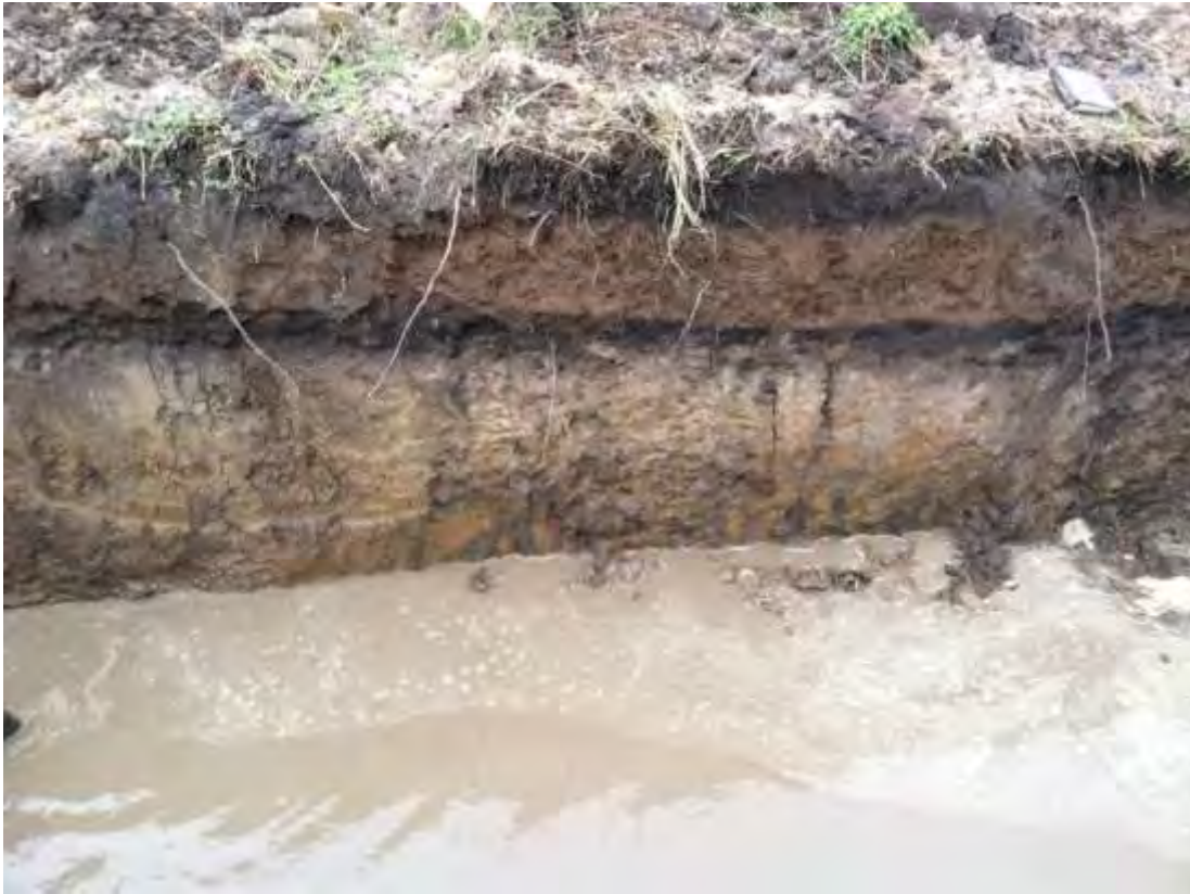
Ron's favorite pit of the contest! (Mapped as Coyne L) Alluvium over windblown sand (with a little organic at surface), over a truncated paleosol formed in glacio-lacustrine sediments. Below the water level was outwash.
