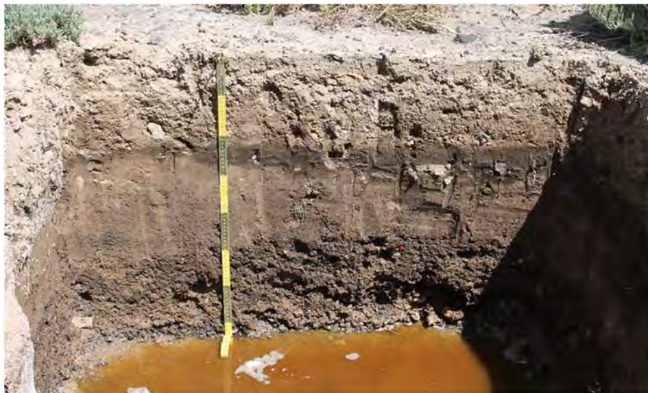
Profile of a soil formed in human transported material (rubble from the 1985 Mexico City earthquake)
